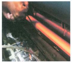
Verify the rod in each die cut area is securely snapped under each retaining bolt head on the cylinder
