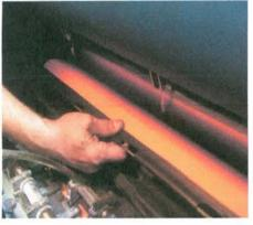
Use the Heidelberg "J" tool to gently apply downward pressure on the stainless steel rod, starting with the center three loops, middle loop first, then the loop to the right of the middle, then the loop to the left of middle, then finally install the "outer" two loops, until the stainless steel rod is securely snapped behind the retaining bolts.
