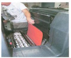
Continue to rotate the cylinder until the elastic loop is resting on the outer edge of the cylinder
