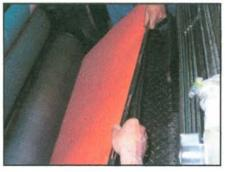
Pick up the jacket by the black elastic loops/steel rod, and slowly rotate the cylinder (continually feeding the jacket so that it wraps the cylinder in a tight and square/true manner) until you have access the pin holes on the transfer cylinder plate. Turn off the press.
