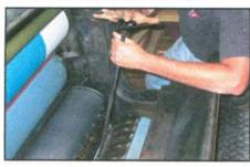
Rotate the transfer cylinder until fully exposing the pin-like bolt heads which secure the steel rod through the die cut portion of the jacket. Turn off the press.
