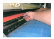
With a pressman on each side, bring the elastic loop/steel rod
