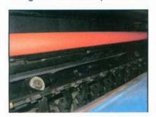
(NOTE: Keep steel rod centered!) over the edge of the flipped up cylinder edge and (continually feeding the jacket so loop under the six (6) spring bolt heads. You should hear an audible click 6 times as the retaining spring is engaged.
